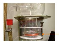
→ Remove the clamping unit (1) at the condenser.
