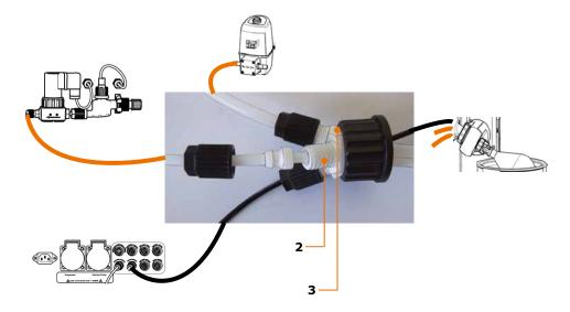
→ Route PTFE tubes and flask sensor into the evaporating flask and secure the multiple screw connection at connection (4) until hand-tight.
