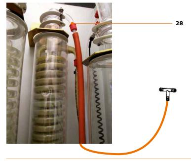
→ Connect the vacuum tube (29) to the evacuation valve of the valve matrix.
