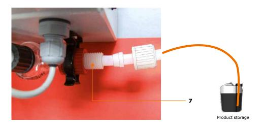
$\rightarrow$  Connect the PTFE tube Ø 6 mm to connection (8) on filter and tighten until hand-tight and run into the product storage vessel.
