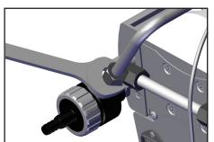
Connect hose to the connection at the inlet of the pump. Tighten union nut first by hand and then tighten one full turn using open ended wrench.
