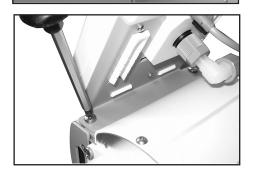
Unscrew both Phillips screws at the fixing plate of the controller.
