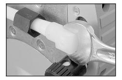
Use open ended wrench (w/f 14) to reconnect hose to elbow fitting.
