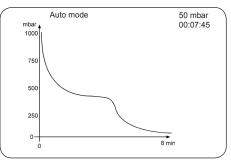
When "Graphic" is selected the display shows a pressure vs. time curve (right screen-shot).
