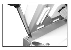
Assemble controller: Use Phillips screw driver to screw both screws through the fixing plate in the square nuts in the housing cover.
