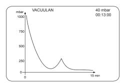
When "Graphic" is selected the display shows a pressure vs. time curve (right screen-shot).
