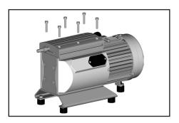
Use a hex key size to loosen the six socket head screws at the pump head and remove the upper housing (housing cover with housing cover insert).
